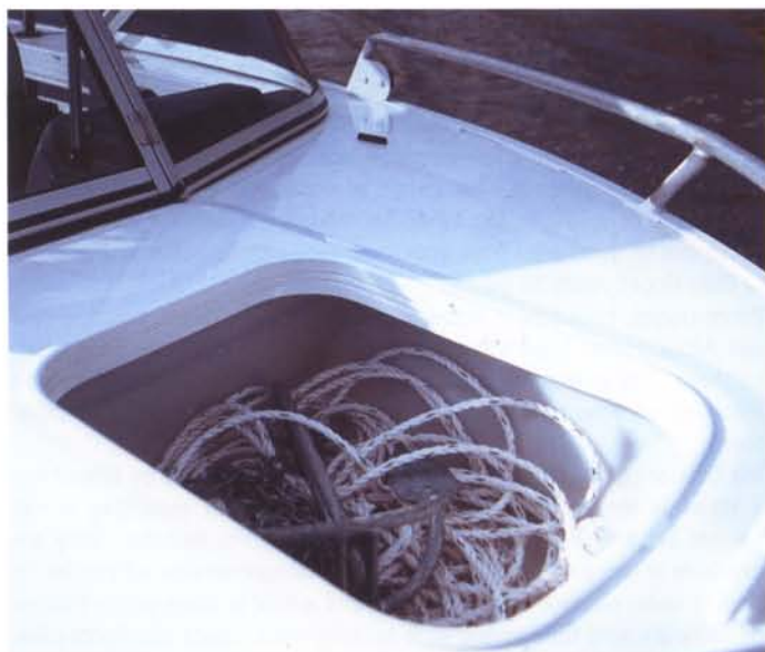
Quintrex's new anchor well with plastic liner.
